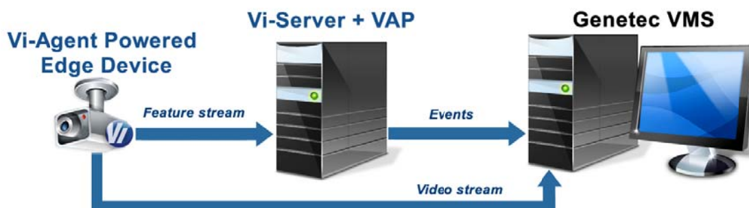
Figure 1-1: Powering Real-Time Analytics with Vi-Agent Embedded IP Cameras
