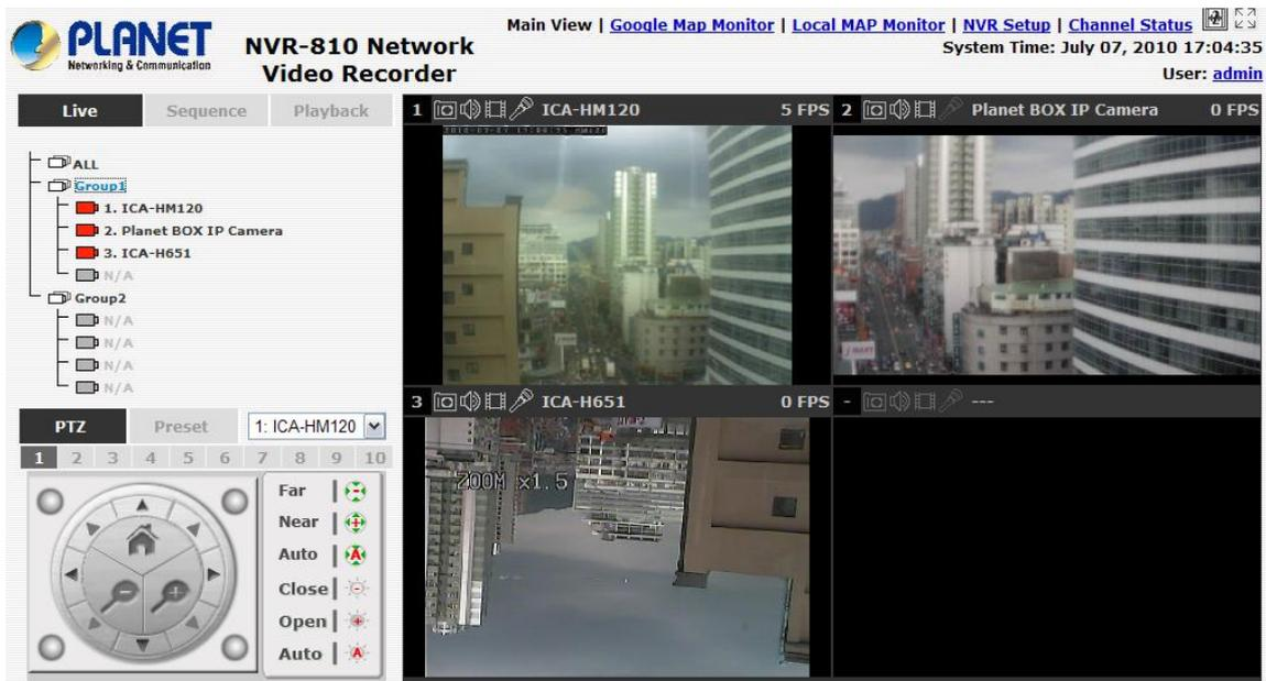
The 8 channel NVR comes with a 8-video split window view with one video displays on a larger window. Select a channel from the drop-down menu to display its video on the larger split window. You can also double-click on any of the smaller one to display its video to the larger window.
